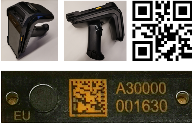
Figure 4: The Zebra RFD40 which can scan both RFID tags and QR codes, and examples of an RFID-tag and QR code.
