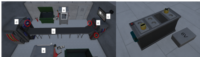
Figure 2: Figure 2: previsualization of the virtual environment volumes (left figure) and an example of a battery model (right figure). (a) module generator, (b) conveyer belt, (c) information panel, (d) entry of the conveyer belt, (e) exit of the conveyer belt.
